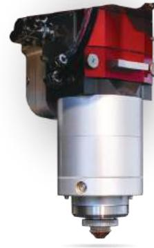
The highly efficient IPG laser source, featuring excellent beam quality and low electric consumption, is housed in an air-conditioned and sealed NEMA 12 cabinet for guaranteed operation even in the harshest of environments. The solid-state reliability of the IPG source virtually eliminates costly maintenance required by competitive laser models.
