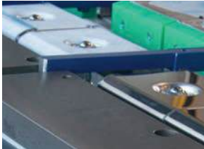
Bottom beam blade with finger grooves
